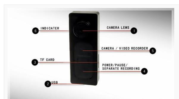
Note: Press 4,5 key to reset (when the machine encounter crash or not charging procedures disorder, please press two keys at the same time to reset)
